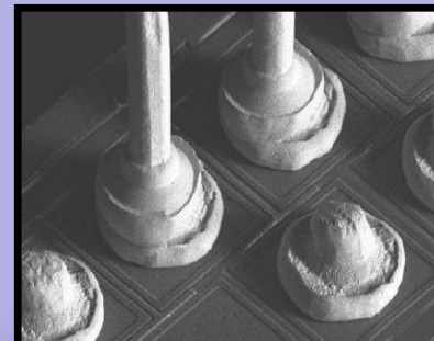
Compound Gold Ball and Aluminum Wedge Bonds
